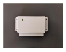
Ambient temperature Ambient humidity String Voltage 0~300V String current 0~400A Digital inputs: 4, isolated
